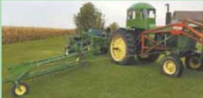
Roadside Rake Pulls Hay Out Of Ditches
