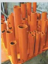
Gene Boehler, Farmersville, III.: "I needed a better way to store tools while at the same time keeping them readily accessible, so I put several short pieces of steel pipe and tubing to good use. They're in various sizes and measure from 6 to 12 in. long. I placed the pipes and tubing in rows about 1 1/2 in. apart. Then I welded them to an 18 by 20-in. base made from 1/8-in. thick steel plate that forms a base, then painted everything bright orange.
