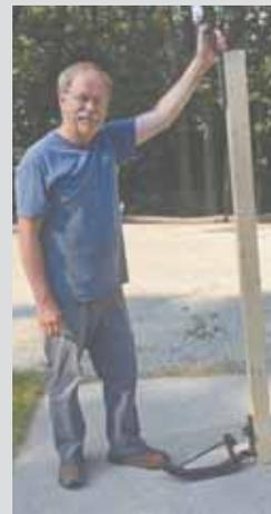
Brush puller consists of two parts that attach to a 2 by 4 with 4 bolts.
