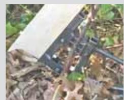
Jaws on puller grab tightly onto stem as the puller is rocked back, pulling brush out by the roots.
