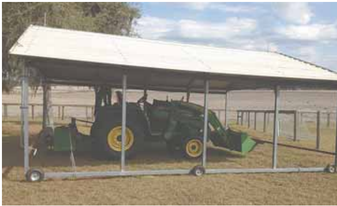
Chains at the front and back of tractor attach to base of carport, where Weller also attached six 8-in. wheels to act as “bumpers” while moving across rough terrain.
