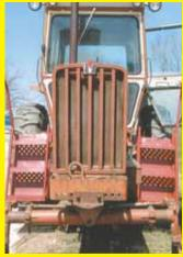
After injuring my rotator cuff, my son Royce installed steps on both sides of my IH tractor so I could get up into the cab. He got the steps off a 6620 Deere combine and welded brackets to the frame of the tractor to support them. Each set is held on by just 3 bolts so they can be easily removed if the tractor needs to be worked on. (Eldon Turner, 76748 Fairview Rd., Anita, Iowa 50020)
