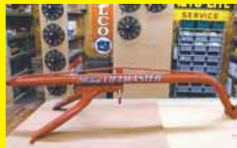
hook on the lifting end swivels and also rotates 360 degrees. The 3-pt. bracket is adjustable both for height and reach. I restore old Chevy pickups and use my Liftmaster like a crane to pick up 6-cyl. engines.
