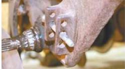
Kit lets you tighten loose seed boot mounts on Deere no-till drills. It includes drill bits and a drill fixture that installs between cast mount ears (above). Worn bolt holes are bored out and new bushings installed.
