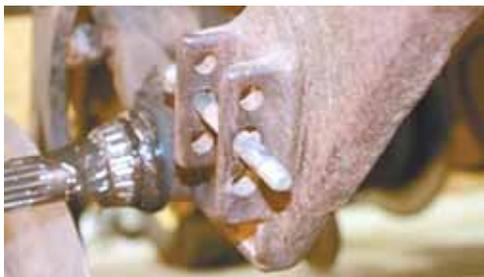
**Kit lets you tighten loose seed boot mounts on Deere no-till drills. It includes drill bits and a drill fixture that installs between cast mount ears (above). Worn bolt holes are bored out and new bushings installed.**
