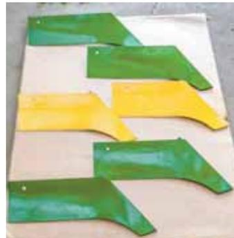
**Steve Rea makes plow shares and other plow and tillage parts the old fashioned way, using a home-built forge and press.**
