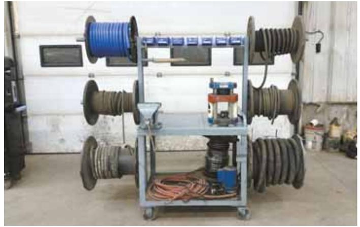
**Rolling repair table has a vise bolted down on one side and a hydraulic press for installing new tips on the other side. A motor to drive the press is stored underneath.**
