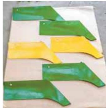
**Steve Rea makes plow shares and other plow and tillage parts the old fashioned way, using a home-built forge and press.**
