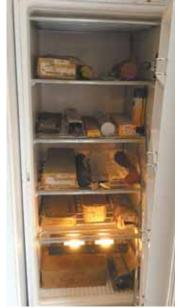
Needing a place to keep his welding rods dry, Doug Clark made this cheap storage cabinet out of an old upright freezer.
