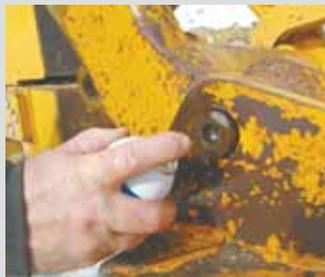
you need is a heavy-duty engine degreaser and a rust buster product such as PB Blaster. First, remove the grease zerk and spray the engine degreaser into the grease cavity. Give the degreaser a few minutes to begin to dissolve the solidified grease, then apply again. Repeat the process until the degreaser flows back out clean.
