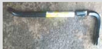
**Tim Glick, Oley, Penn.:** "I made a 3/4-in. hex driver to insert into my 3/4-in. socket by cutting a 3-in. section out of a new crowbar. Stores don't carry a hex driver this large. I needed one to remove a pair of hex-shaped oil drain plugs on the front axle differential on my mechanical front-wheel drive tractor. I paid \$12 for the crowbar. Now I've got a new hex driver, and I can use the rest of the crowbar as a prybar."
