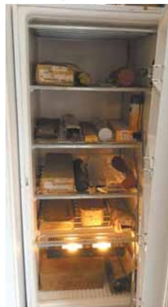
Needing a place to keep his welding rods dry, Doug Clark made this cheap storage cabinet out of an old upright freezer.
