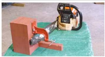
Wood block fitted with screw clamp holds chainsaw's bar steady for chain tightening and hand sharpening.
