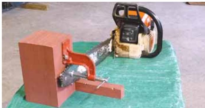
Wood block fitted with screw clamp holds chainsaw’s bar steady for chain tightening and hand sharpening.
