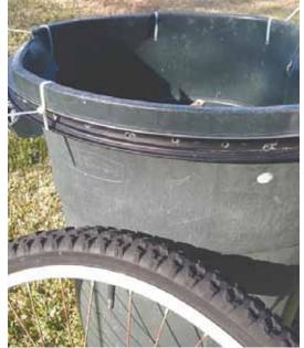
Photo shows a 26in. bike wheel rim zip-tied to the rim of a Rubbermaid trash barrel.
