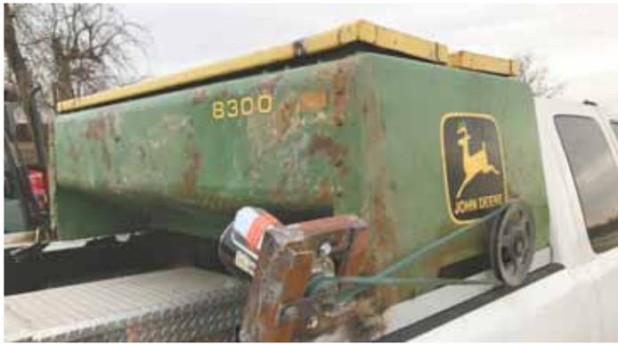
Pickup-mounted cake feeder was built from an old grain drill box. Burrell installed a 6-in. dia. auger just above drill's sloped floor and uses a car starter and a belt to drive it.
