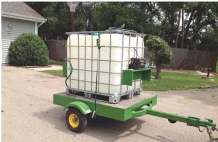
A 25-ft. long garden hose, equipped with a sprinkler attachment, hooks up to a 12-volt pump on one side of tote. A 12-volt battery is mounted on the other side.
