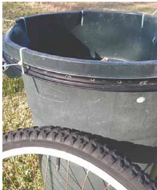
Photo shows a 26-in. bike wheel rim zip-tied to the rim of a Rubbermaid trash barrel.
