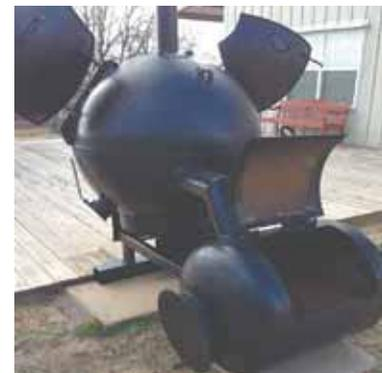
Heat and smoke from firebox is ducted through two 6-in. pipes to main smoker.
