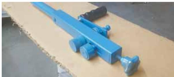
Hand-cranked roller consists of a 1-in. sq. steel tube with 2 steel rollers.
