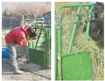
To keep calves from climbing into his big bale feeder, Thomas welded a pair of 3/8-in. rebars across each stanchion, just below the feeder's top rail.
