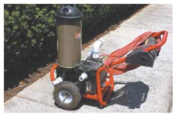
Browning mounted the pump and canister filter off a commercial swimming pool cleaner on the frame of an old pressure washer. "The pool cleaner's big 10-micron filter removes most of the impurities in the water," he says.
