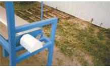
Operator releases a latch at one end of trough and grabs a metal rod to tip trough forward. It automatically relatches when tipped back into place.
