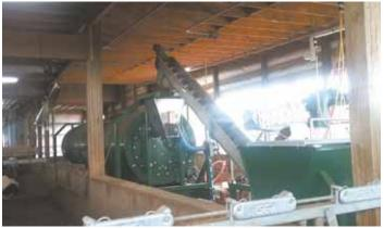
Dorrich Dairy uses compost made from manure to bed their cattle. A large rotating drum receives material and a conveyor at the opposite end removes it.
