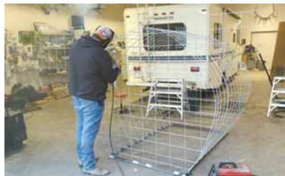
**Barabash built blind’s frame by bending metal hog panels and welding them to a rectangular angle iron base.**
