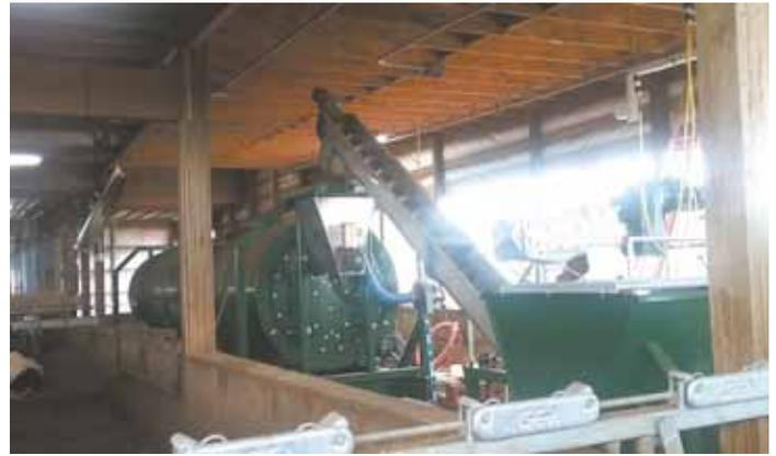
**Dorrich Dairy uses compost made from manure to bed their cattle. A large rotating drum receives material and a conveyor at the opposite end removes it.**
