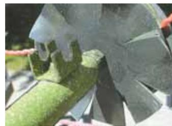
Slotted metal cutter plate replaces trimmer line cutting guard to keep grass from wrapping.
