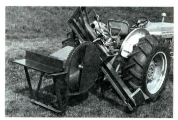
Saw runs off the tractor's pto and the wood splitter off the hydraulic system. Saws logs up to 12 in. in dia. and splits logs up to 26 in. long.
