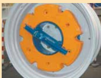
A mounting plate permanently mounts to the wheel studs. When weight is needed, it slips over the mounting plate and is held in place by a hand-turned bracket that extends across both sides. A removable handle is used to turn the lock-down bracket.
