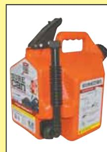
**SureCan has a thumb trigger on top and a flexible rotating spout at bottom. Pushing down on trigger opens a vent and valve at the same time to dispense fuel out bottom of can.**
