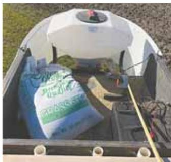
**A separate 12-volt battery is used to power the spreader.**
