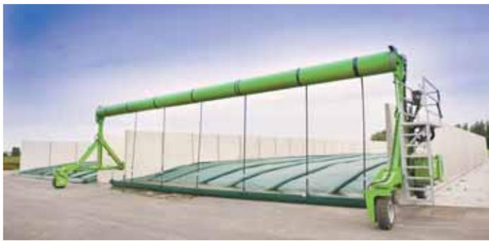
Retractable bunker cover system uses a set of A-frame gantries that run outside bunker walls, quickly unrolling or rolling up a weatherproof cover over silage. It's held in place by filling overlying hoses with water.
