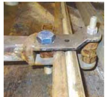
A big bolt runs through yoke and serves as a pivot point. Pulling down on handle causes another bolt with nuts on it to push against pipe to bend it inward.
