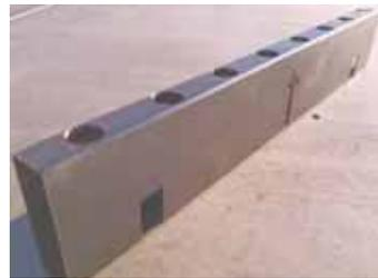
Pipes fit through holes spaced several inches apart at top and bottom of template.
