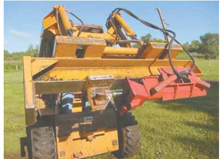
Mark Majerus made use of the auxiliary hydraulics on his Case skid loader to build this hands-free log splitter. It can be used as a "thumb" to pick up wood to split or load it onto a pile.
