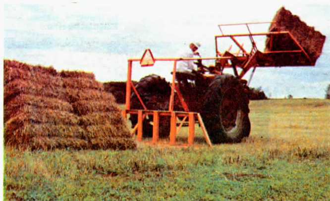
Zimmerman says his bale forks for front-end loader and rear 3-pt. can pick up six stacks - a total of 36 bales - at once.
