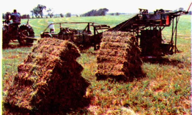
Automatic stacker tows directly behind baler. A ground-driven wheel powers deflector plates and sorting arms that put bales in triangular-shaped stacks.
