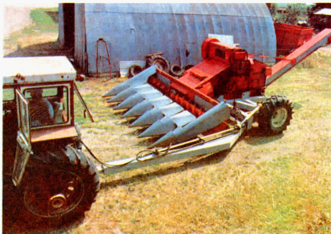
Roger Montag's cart converts self-propelled Uni-Systems to pull-type. Model shown is equipped with a husker bed and 6-row head and is pulled by an IH 856 tractor.
