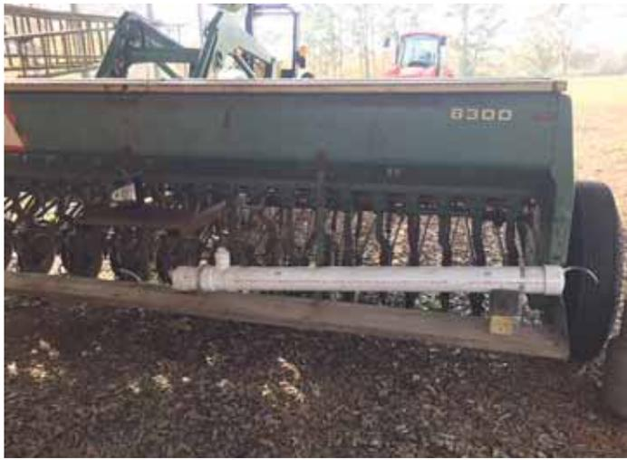
A small 12-volt air compressor pressurizes a 4-ft. length of 4-in. dia. pvc tubing. The homemade foam marker mounts on back of Ruffin's grain drill.
