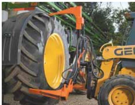
Skid loader-mounted Tire Grabber uses 3 telescoping arms attached to plates mounted on a hub. A hydraulic cylinder extends the arms in unison.
