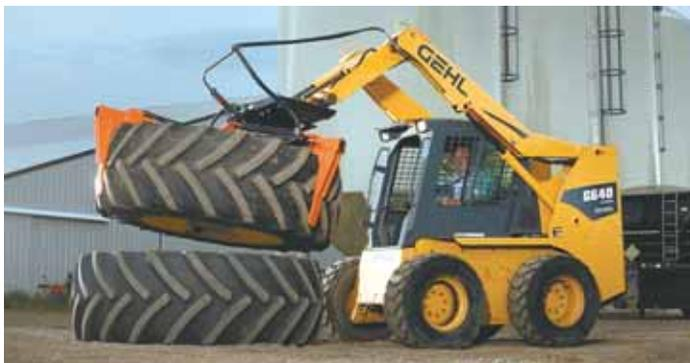
Tire Grabber can lay a tire flat on the ground or on a stack.
