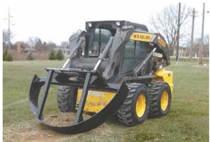
Half circle design of Myron Isaacson's Dream Bucket makes it easy to dig a ditch, level a pile, or fill a hole.
