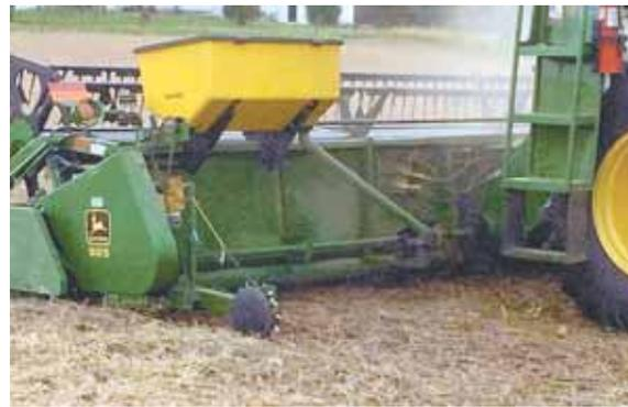
Simple ground drive unit on this soybean header ensures that seed is only spread when the header is down and moving through the field.
