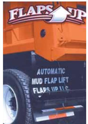
An electric motor control automatically raises mud flaps whenever truck is put in reverse. Driver pushes an in-cab switch to let flaps back down.
