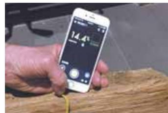
“Moisture readings don't actually show up on the **Ryobi**. The meter is a twin prong device that fits in the palm of my hand. A cable from it plugs into the phone jack on my cellphone. To get a moisture reading, I plug it in, pull up an app on my phone (downloaded from **Ryobi**) and select the type of wood.
