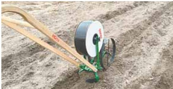
Hoss Tools’ new drip irrigation tape layer attaches to the company’s double wheel hoe, making it easy to lay down and bury drip tape in one pass.
