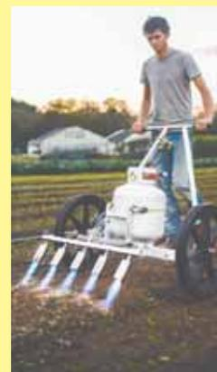
Riding on 2 wheels, the Pyroweeder has burners on front and can carry either one or two propane tanks.
