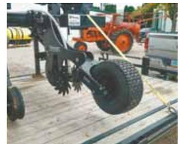
Strip Till For You designs strip-till, no-till and fertilizer application equipment for customers. Photo at right shows a Yetter strip freshener converted for interseeding, and rubber tire packing wheels.
