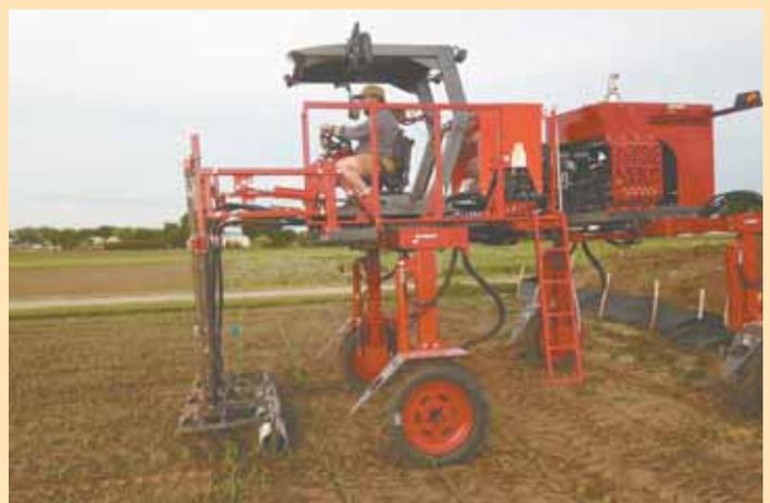
They mounted a Gandy orbital air seeder with adjustable length drops and seed dispersers on the sprayer.
