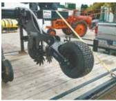
Strip Till For You designs strip-till, no-till and fertilizer application equipment for customers. Photo at right shows a Yetter strip freshener converted for interseeding, and rubber tire packing wheels.
