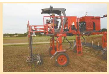
They mounted a Gandy orbital air seeder with adjustable length drops and seed dis-
