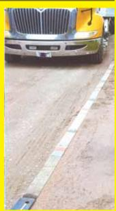
I made this nylon strap gauge so drivers know where to stop when filling their semi trucks as they load grain out of bins. The strap is marked with different spray-painted colors for different trucks. I zip-tied both ends of the strap to chunks of metal that hold the strap down. It can be quickly folded up to move somewhere else. Saves us a lot of time. (Todd Martin, Wayne City, III.)
