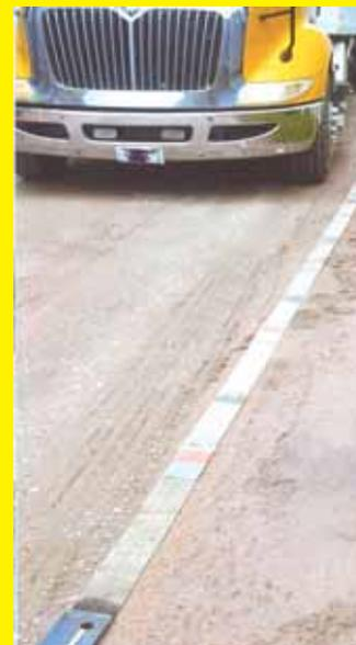
I made this nylon strap gauge so drivers know where to stop when filling their semi trucks as they load grain out of bins. The strap is marked with different spray-painted colors for different trucks. I zip-tied both ends of the strap to chunks of metal that hold the strap down. It can be quickly folded up to move somewhere else. Saves us a lot of time. (**Todd Martin, Wayne City, Ill.**)
