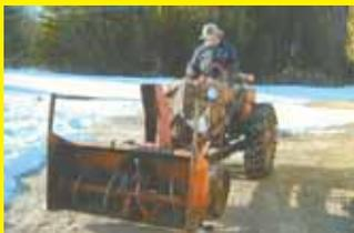
For 34 years I've used my IH Cub tractor to power a 4-ft. wide snowblower I bought used from a local implement dealer. The snowblower is powered by a Wisconsin 2-cyl., electric start engine that mounts on the back of the tractor.
