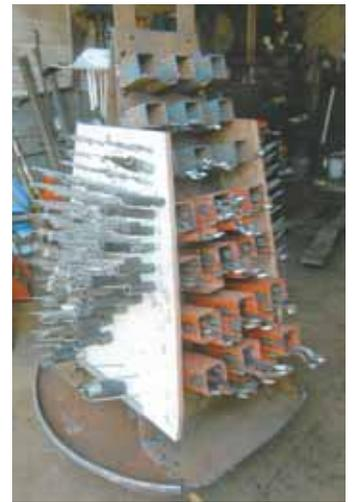
Four-sided Lazy Susan spins on a tandem axle manure spreader wheel and hub that serves as the base.
