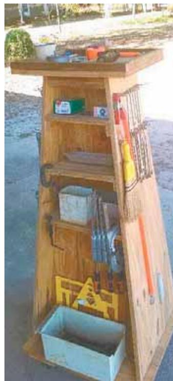
Cabinet sides taper from 22-in. edges at the bottom to 10-in. edges at the top. The taper makes cabinet hard to tip.
