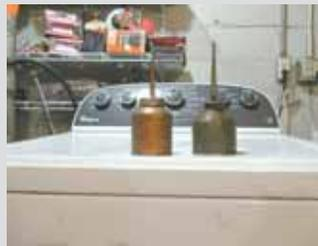
**Ken Ladd, Minneapolis, Minn.:** "My cousin and I were trying to figure out how to store and apply our home brew mix of 50-50 automatic transmission fluid and acetone that we use as a penetrating oil to loosen up rusted nuts. I went on eBay and found some inexpensive vintage oil cans with spouts. The can shown at left in the photo has no gasket that could leak fluid. The other can does have a gasket, but hopefully it will stand up to use."
