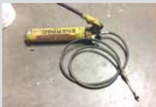
help. Then someone suggested that I adapt a zerk fitting to the hose on a Porta-Power, so I attached the Porta-Power's 3,000-lb. psi flexible hose to a grease zerk connector. It worked.
