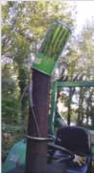
"To solve the problem, I came up with what I call my 'spring-loaded asparagus can cover.' I've used this idea on all 3 of my tractors equipped with vertical exhaust stacks, and it works great. However, whenever I need to use the tractor for an extended period of time I remove the can to keep fumes out of my face."
