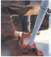
Benoit added 3 homemade spacers to raise the back end of his posi track skid loader, allowing him to work on the tracks.
