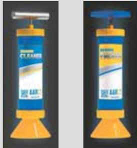
The bearing cleaner consists of a plunger inside a cylinder-shaped chamber; a screw-on, cone-shaped plastic base; and a small black cone. The operator fills chamber at least 3 in. deep with cleaning solvent. He then places the cone over the bearing and pushes down on the plunger to flush all the grease out of the bearing. At the same time, the cleaning solvent will be forced up through the bearing’s rollers.
