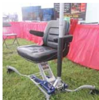
**Pumping on hydraulic floor jack handle lifts operator from kneeling level up to a sitting position.**
