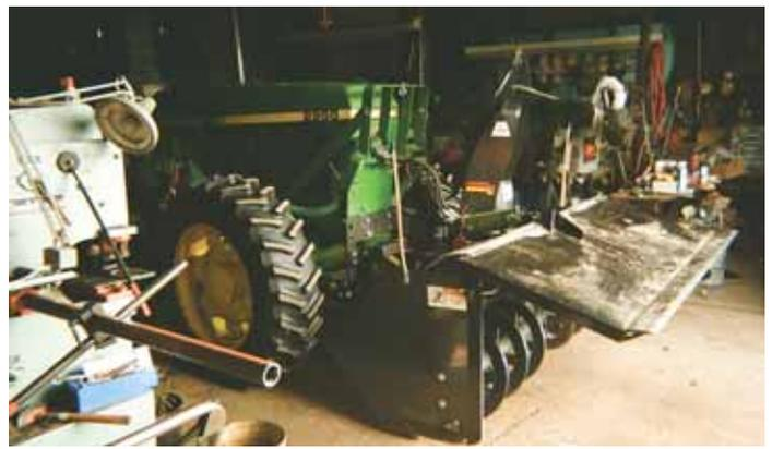
**Hinged, hydraulic-operated "door" on front of snowblower is raised up or down by pulling a lever in the cab. With door all the way down Krueger can push slush around without getting it into the auger. To use the snowblower again he just raises the door.**
