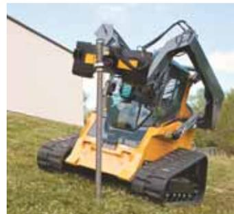
**Built-in manifold regulates hydraulic flow to driver as it pounds post into ground.**
