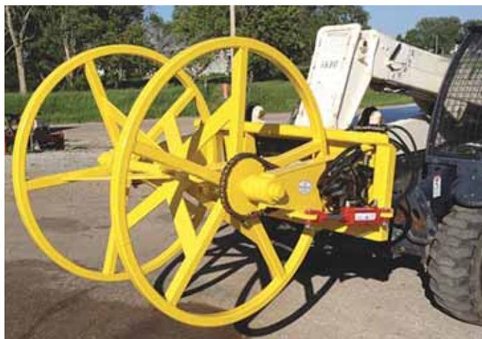
Giant wire winder is chain-driven by a hydraulic motor. TC Machine says it works great to wind up plastic silo bags.
