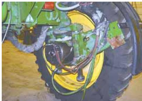
Photo above and at left shows Deere 4930 sprayer being fitted with new ATC electric drive wheel motors.
