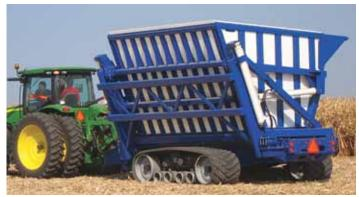
Side dump grain cart is equipped with 4 large hydraulic cylinders – 2 to raise and lower the box and 2 to tilt and dump it. There's no pto, augers or flighting to wear out.
